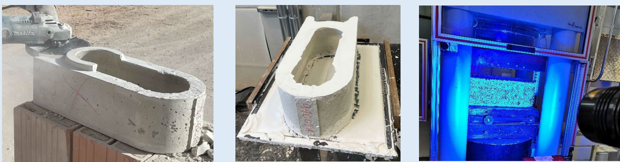
Figure 2: TwistBlock preparation for overall compressive test. Left: cutting off of extensions; middle: application of gypsum; right: compression test
